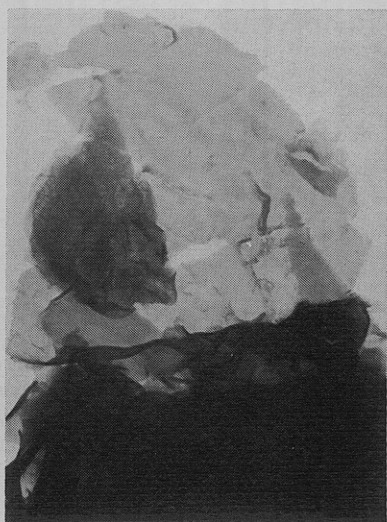
Figure 23. Electron micrograph of debris from selective oxidation for M = 284,000 crystallized at 130.1^\circ for 6 weeks.
