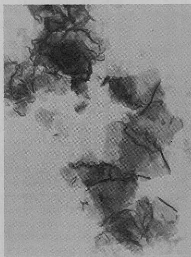
Figure 24. Electron micrograph of debris from selective oxidation for M = 8 \times 10^5 crystallized at 130.1^\circ for 6 weeks.
